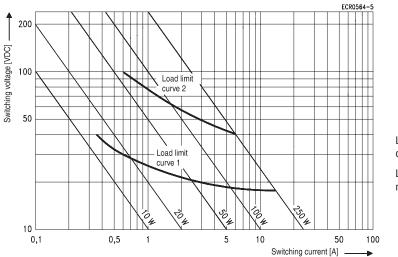
Load limit curve  $1 \triangleq arc$  extinguishes, during transit time (changeover contact)
